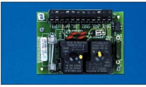
The SB520 enables the SNM800 to drive sounder circuits with higher currents whilst maintaining the reverse polarity integrity line monitoring.
