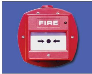
The CP830 is an outdoor MX addressable manual callpoint with programmable status LED. The CP830 is designed for LPCB approvals . The CP830 provides high speed communication to the MX panel of a manual fire alarm.
