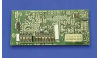
The APM800 is an MX addressable power supply monitoring module which is usually used with the PSM800 power supply module to make an addressable power supply. The APM800 is designed to fix to studs on the top of the PSM800.
